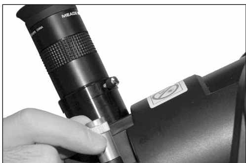
Steps 4 and 6: Insert eyepiece and focus telescope.
