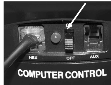
Fig. 11b: Connect the AutoStar handbox and turn on the computer control panel.
