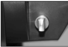
Fig. 4a: Flip mirror control in the "up" position.
