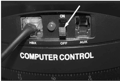
Step 8: Plug in handbox and turn on computer control panel.
